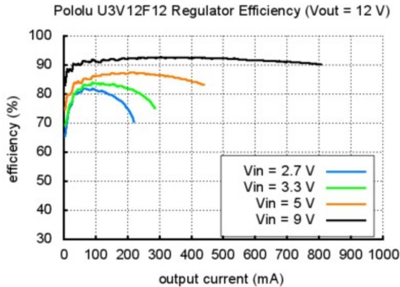
The maximum achievable output current is approximately proportional to the ratio of the input voltage to the output voltage. If the input current exceeds the switch current limit (typically somewhere between 1.4 and 2 A), the output voltage will begin to drop. Additionally, the maximum output current can depend on other factors, including the ambient temperature, air flow, and heat sinking.
